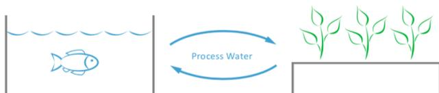
Figure 1. Aquaponics: coupled (one-loop) system
