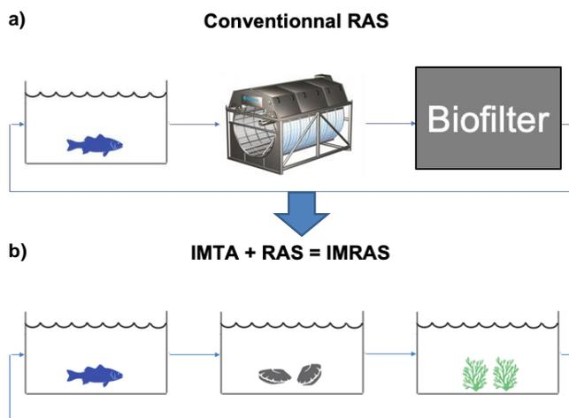
Figure 1. (a) Standard RAS with fish tank, mechanical filter and biofilter, (b) IMRAS with fish tank, shellfish tank which replace the mechanical filter and seaweed tank which replace the biofilter
